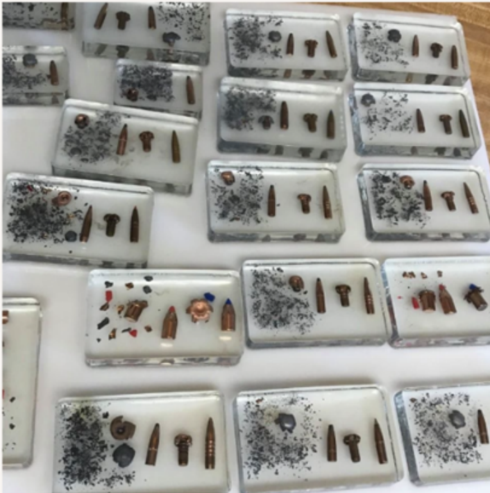
An assortment of lead bullets showing shot fracturing next to similar fired copper variants
